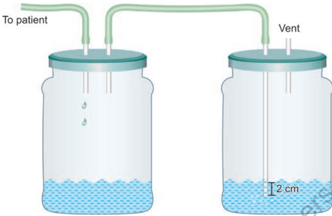
Fig. 7 Two-bottle drainage system
